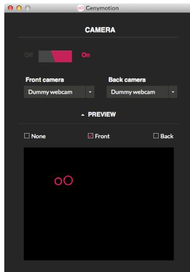
The video stream can come from a dummy camera or a real physical webcam connected or integrated into your computer.
